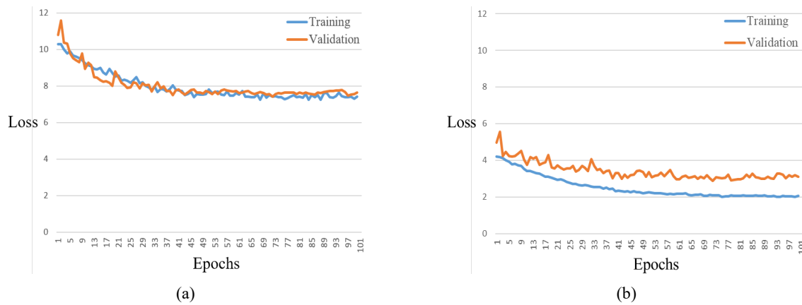
Fig.6. The training history of YOLOv4 (a) without Cosine Annealing LR, (b) with Cosine Annealing LR.
